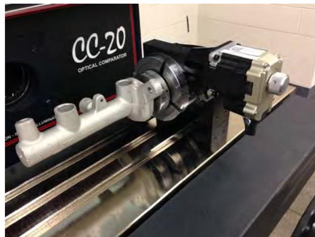
**Helix motion** – allows off-axis measurement of threads, gears, and gear cutting tool hobs by rotating the part so that the features are presented correctly to the optics and measured normal to the part axis.
